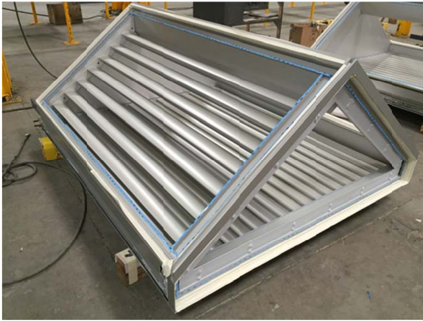
Curtain Wall Unit in Fabrication
